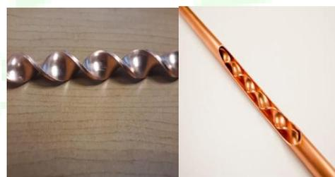
(a) Twisted Tape Turbulator (b) proto type Turbulator
