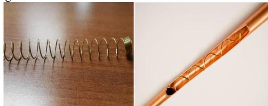
(a) Spring Turbulator (b) Tube wall with Ball Turbulator
