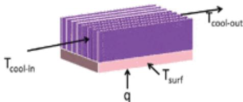
Fig. 1. Simple heat sink
