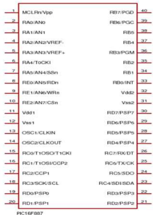
Fig.10. PIN DIAGRAM OF PIC 16F887
