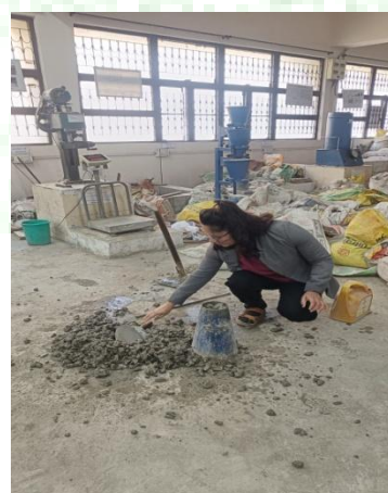
Fig:6 Concrete Slump Test Procedure
