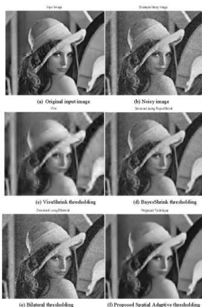
Figure shows the image denoising using various thresholding methods. From figure, the proposed spatial adaptive thresholding algorithm provides better performance compared with thresholding methods like VisuShrink, BayesShrink, and Bilateral threshold providing a better PSNR and MSE values.
