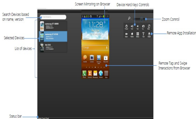
Figure 3 Remote monitoring and controlling of devices on browser
