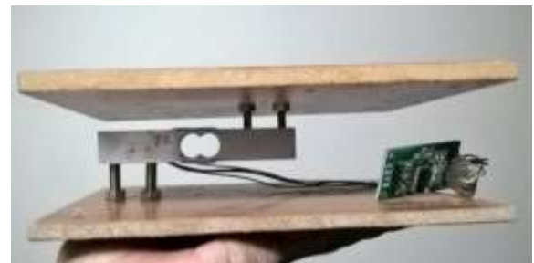
Fig.4. Loadcell and HX711 Arrangement
