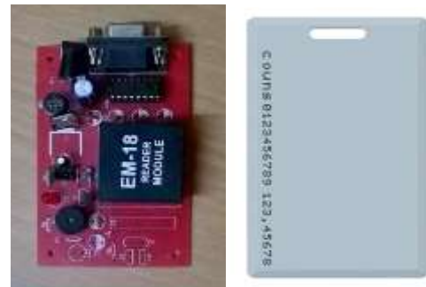
Fig.3. EM-18 RFID Reader and Passive Card
