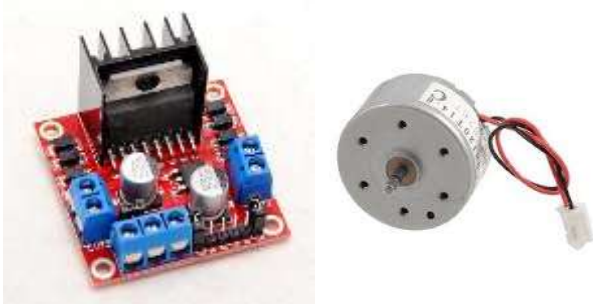
Fig.7. DC Motor and L298N Driver
