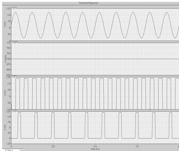
Fig. 10 Transient response of the Comparator (semi-dynamic Latch)
