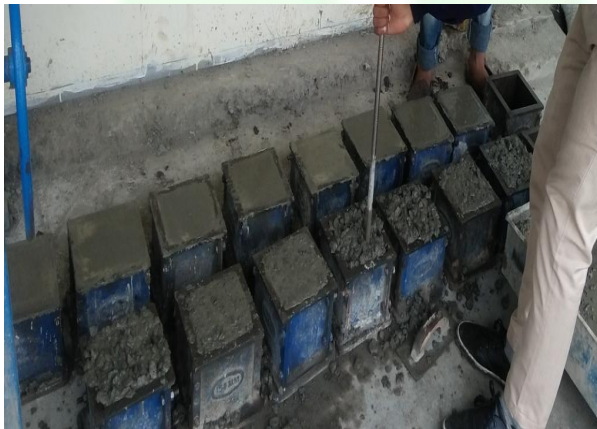
Image 1: Filling up the Concrete moulds
