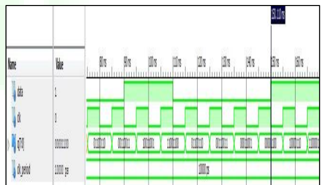
Figure: 3 Simulation result for parallel in serial out shift register
