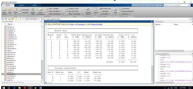
Figure 4: Results window shows the updated Branch data and voltage constraints for IEEE-9-Power System Bus
