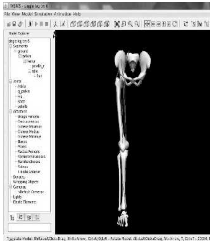
Figure 1 (A): Proposed right leg model in MSMS with rigid body segments, joints and 12 virtual muscles.
