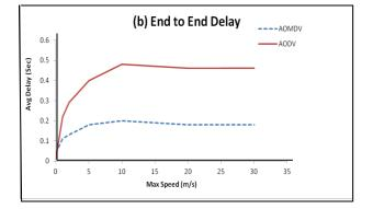
With the increasing traffic load, the burden of intermediate nodes will be aggravated and in turn resulting the failure of resource reserving.. By using multipath method, our proposed method can balance the traffic load through sending data along different paths which is responsible for reducing the packets collision.
