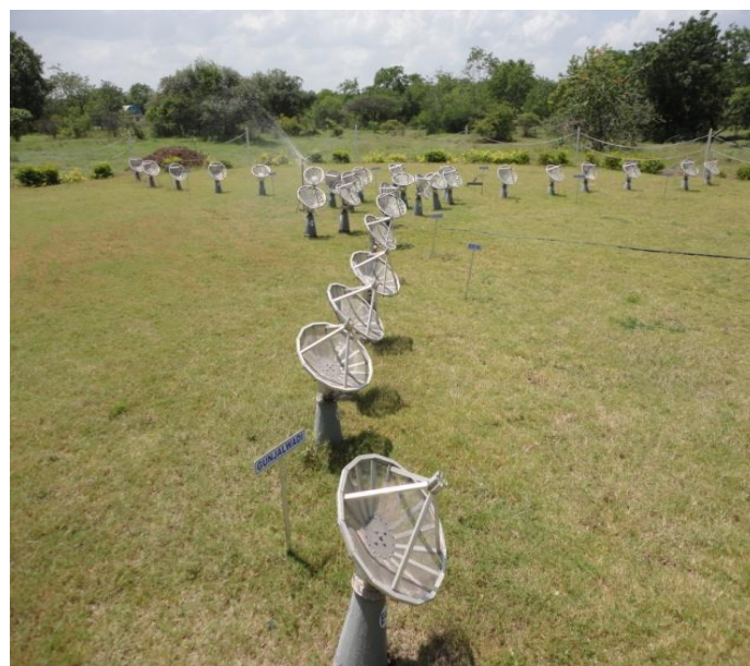
Picture 1: Model showing positions of 30 antennas erected in an imaginary circle of 25km diameter.
