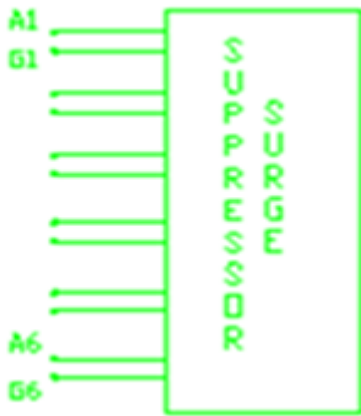
Fig.4: Surge Suppressor working as the protection module. The surge currents and spikes of currents are suppressed by this module making these spikes smoother to avoid any triggering.
