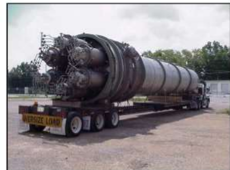
Figure 1: shell and tube heat exchanger made by Addison Fabricators Inc., Addison, Alabama, USA (8000 tubes/90 tonnes).
