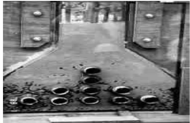
Figure 2.1 Small pipes used as obstacles in formwork (Okamura, 1997).
